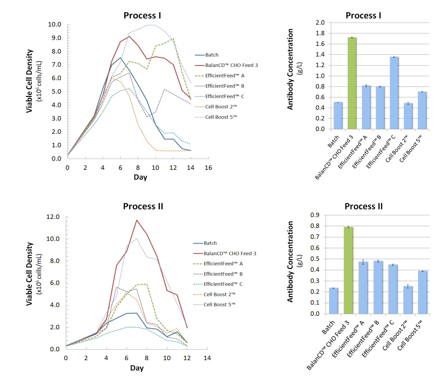
The resulting feed, BalanCD<sup>™</sup> CHO Feed 3, worked well with both processes.
