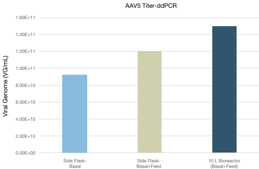
Figure 4. Verification of the BalanCD HEK293 Viral Feed performance on improving the production of AAV5 in 10 L bioreactor scale. HEK293 suspension cells (cell line 2) were seeded at density of 0.8 \times 10^6 cell/mL in 8.3 L culture volume in 10 L bioreactor (XDR10 bioreactor). BalanCD HEK293 Viral Feed was added at 12% v/v at 24 hr post transfection. Titer was measured using ddPCR.
