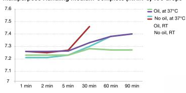
pH maintained between the ideal range of 7.2–7.4 at room temperature and in an incubator under oil.
