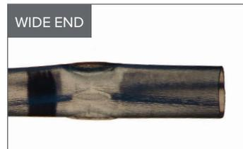
Example of a under-sealed CryoTip
