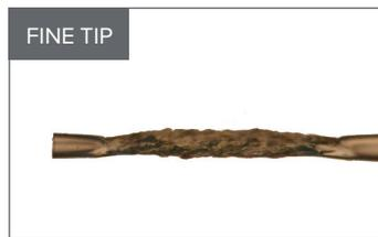
Example of an over-sealed CryoTip
