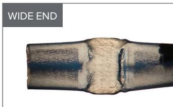
Example of a good sealed CryoTip
