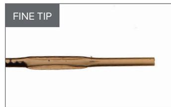
Example of a under-sealed CryoTip
