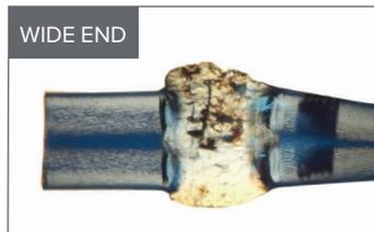
Example of an over-sealed CryoTip
