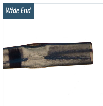
Example of an under-sealed CryoTip
