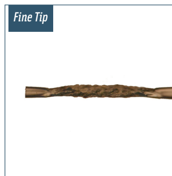
Example of an over-sealed CryoTip
