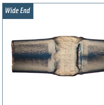
Example of a good sealed CryoTip
