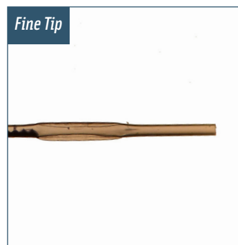
Example of an under-sealed CryoTip
