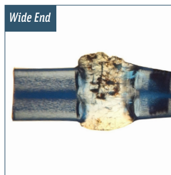
Example of an over-sealed CryoTip
