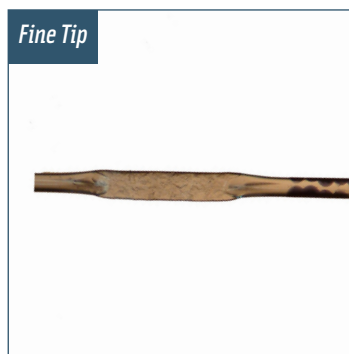
Example of a good sealed CryoTip
