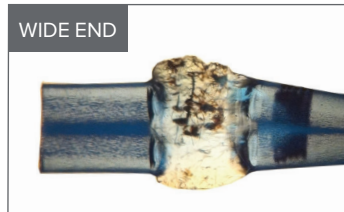
Example of an over-sealed CryoTip
