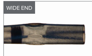
Example of a under-sealed CryoTip
