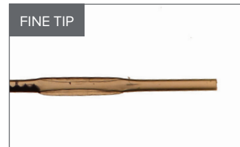
Example of a under-sealed CryoTip
