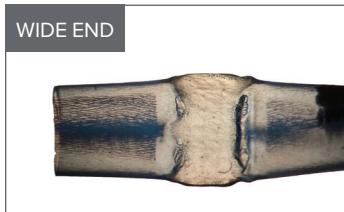
Example of a good sealed CryoTip
