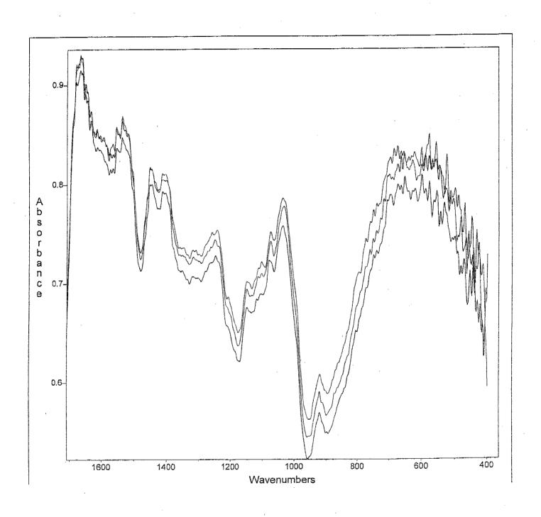
**Figure 2. FTIR Method Reproducibility.** Three independent samples of the same lot of hydrolysate were analyzed to demonstate the reproducibility of the FTIR analysis method. The samples were analyzed at a 20% sample:KBr ratio.
