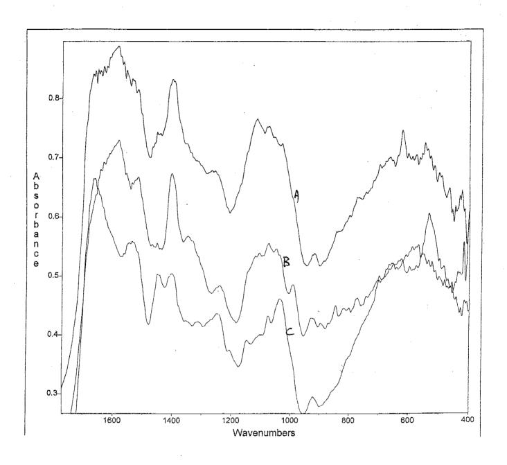
**Figure 4. Distinguishing Various Hydrolysates.** This figure demonstrates how an FTIR method can effectively distinguish between different hydrolysates. The spectra acquired from hydrolysates of three different non-animal sources are shown.
