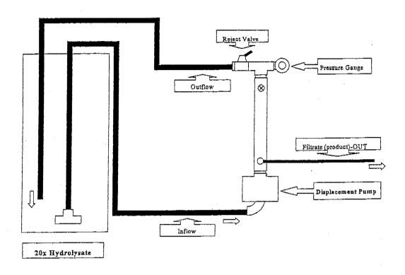
**Figure 5. Ultrafiltration of Hydrolysates.** A concentrated solution of dissolved hydrolysates may be ultrafiltered and subsequently dried for use in culture media. A 10,000 MWCO membrane is most commonly used
