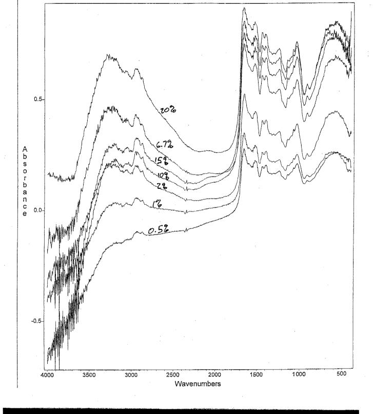
**Figure 1. FTIR Method Development.** Because of the complex composition of hydrolysates, special methods were developed for Diffuse-Reflectance FTIR matching. Besides customizing the matching algorithm, the sample:KBr ratio was optimized to best exploit the special features of hydrolysate spectra. The figure demonstrates the effects of adjusting the sample:KBr ratio over a range from 0.5-20%.
