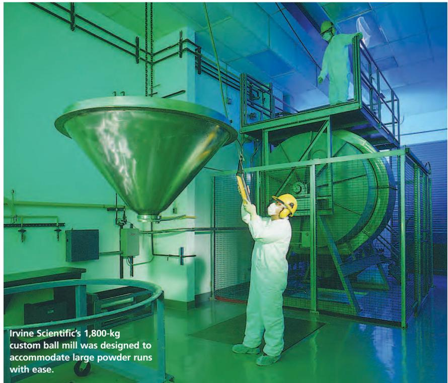
Irvine Scientific's 1,800-kg custom ball mill was designed to accommodate large powder runs with ease.
