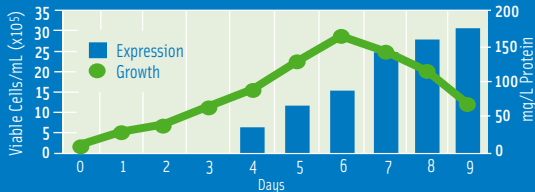
Figure 1. Growth and Expression in Shaker Culture. CHO Line 2 (dhfr selection). 30 mL culture in 125 mL shaker flask at 160 RPM. Protein determination by HPLC.
